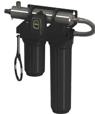
The wall mounted filtration unit is designed to accommodate flow rates up to 8 GPM and handle a maximum pressure of 120 psi at 113°F (45°C) maximum temperature. Standard inlet and outlet connections are 1” NPT. Standard head unit is reinforced polypropylene. Standard O-ring is EPDM.
