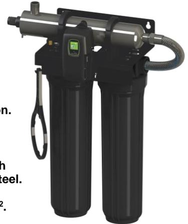
The wall mounted filtration unit is designed to accommodate flow rates up to 15 GPM and handle a maximum pressure of 120 psi at 113°F (45°C) maximum temperature. Standard inlet and outlet connections are 1" NPT. Standard head unit is reinforced polypropylene. Standard O-ring is EPDM.
