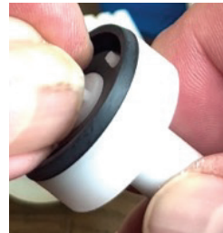
The solenoid pulls the piston down, which cause the diaphragm to allow debris to pass as large as a 1/4"
