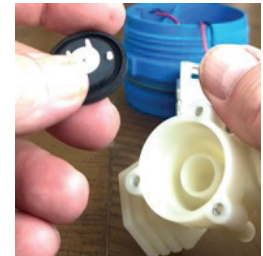
The diaphragm seals against the fitting by pressing against the edge
